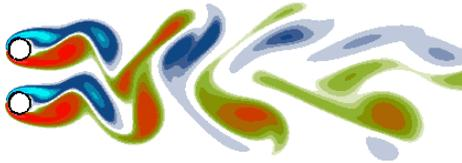
Figure 4: Flow past two circular cylinders placed normal to the oncoming flow using the Chimera method for  $Re=100$ .
