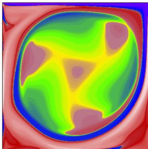
Figure 1: Vortical structures inside a square lid-driven cavity for  $Re=10,000$ .
