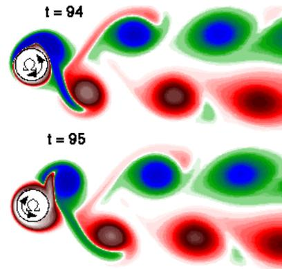
Figure 2: Flow past a circular cylinder executing rotary oscillation for  $Re=150$ .
