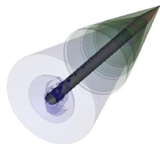
Figure 3: Pressure contour surfaces for hypersonic transition over a tangent-ogive body at Mach no. 4,  $Re=1.12 \times 10^6$ .
